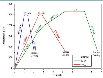
Figure 1. Temperature versus time plots for conventional, microwave and vacuum sintering operations.
