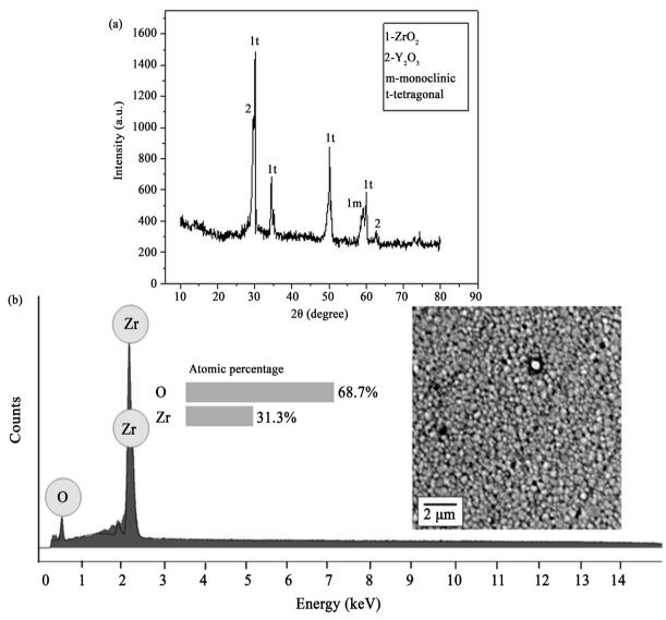
Figure 5. Typical (a) XRD plot and (b) EDX pattern in association with SEM image (shown in inset) of sintered nano-YSZ specimen.
