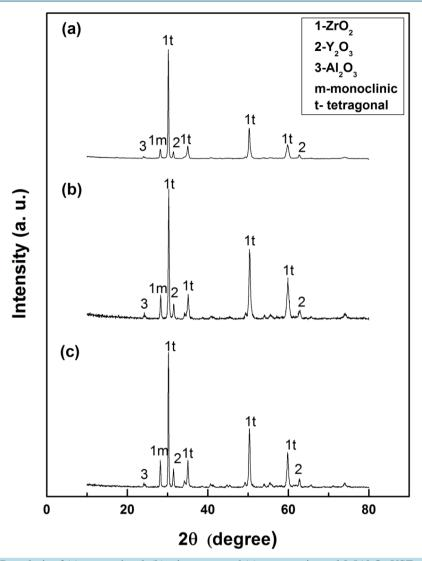
Figure 3. XRD analysis of (a) conventional, (b) microwave and (c) vacuum sintered 0.5Al<sub>2</sub>O<sub>3</sub>-YSZ specimens.
