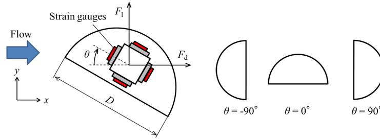
**Figure 2.** Semi-circular cylinder and strain gauges.
