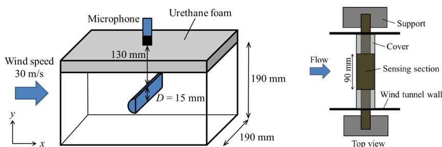
**Figure 1.** Experimental setup.
