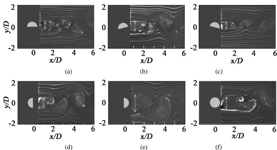
**Figure 8.** Smoke-wire flow visualizations of flow around circular and semi-circular cylinders. (a)  $\theta = 0$  degree; (b)  $\theta = -15$  degree; (c)  $\theta = 15$  degrees; (d)  $\theta = -90$  degrees; (e)  $\theta = 90$  degrees; (f) Circular cylinder.
