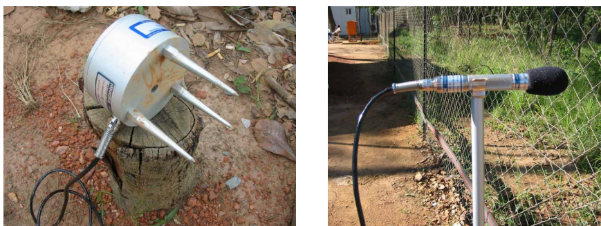
Figure 2. Parts of the calibrated seismographs.
