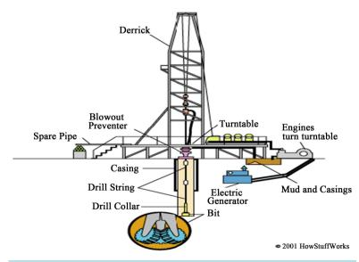
Figure 1. Rotary drilling rig (modified from Craig and Jonathan, 2001).
