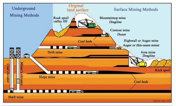
Figure 2. Different coal mining methods. Source: www.worldcoal.org/coal/coal-mining/.
