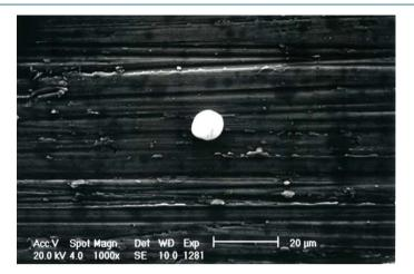
**Figure 4.** Surface appearance of the extracted BMG after 6 weeks implantation. Scanning electron microscopy (SEM), ×1000.
