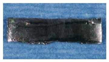
Figure 6. The extracted BMG ribbon. This photo shows the side that had been in contact with the femur.
