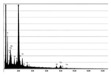
**Figure 5.** Energy dispersive spectroscopy (EDS) of the surface of the BMG after 6 weeks implantation. The constituents of the surface materials included Na and Cl.
