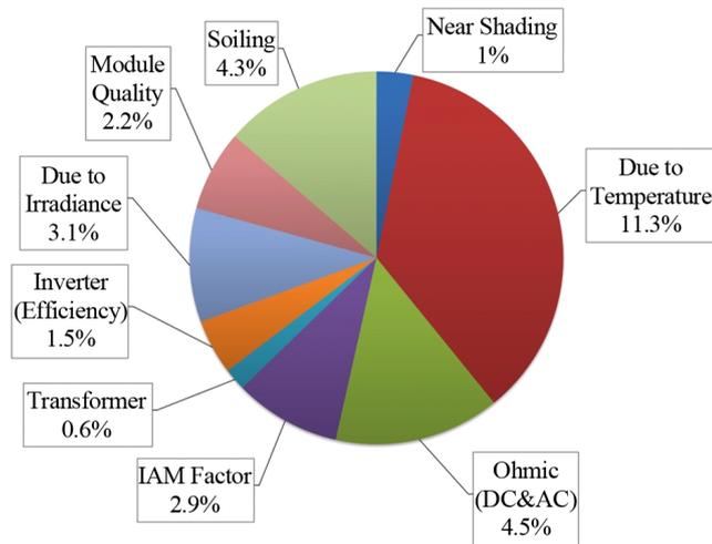
Figure 5. Energy loss profile based on near shading, temperature, irradiance, ohmic, IAM factor, transformer, inverter, soiling and module quality.
