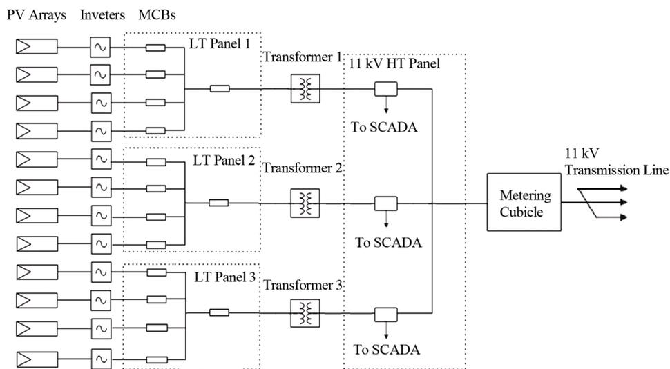
**Figure 1.** Schematic diagram of 3 MW solar power plant at village Yalesandra, Dist. Kolar (Kolar Plant), Karnataka [14].
