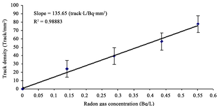
**Figure 3.** Shows the relation between radon gas concentration and track density in standard water samples.
