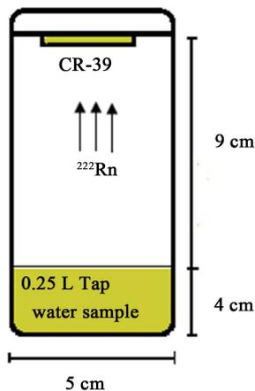
**Figure 2.** Sealed-cup (can) technique use for water samples.
