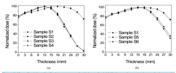
Figure 3. Normalized dose distribution versus sample thickness for 9 MeV electron beam: (a) thermoplastic material (S1) and RTV-530 based samples (S2 - S4); (b) thermoplastic material (S1) and GSP400 based samples (S5, S6).
