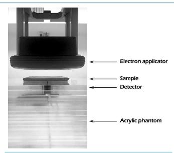
Figure 1. Experimental setup for transmitted dose measurements.
