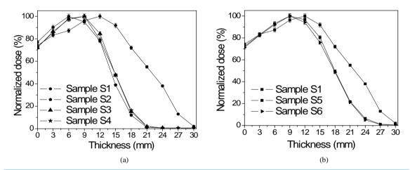
Figure 2. Normalized dose distribution versus sample thickness for 6 MeV electron beam: (a) thermoplastic material (S1) and RTV-530 based samples (S2-S4); (b) thermoplastic material (S1) and GSP400 based samples (S5, S6).
