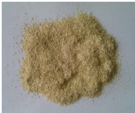
Figure 3. Grinded Luffa fibers of particle size 1.0 .mm.
