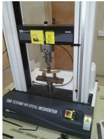
Figure 6. UTS machine Sample loaded for Flexural testing.
