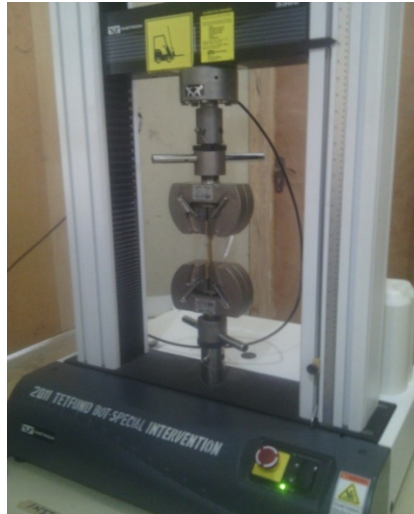
Figure 5. UTS machine sample loaded for tensile.
