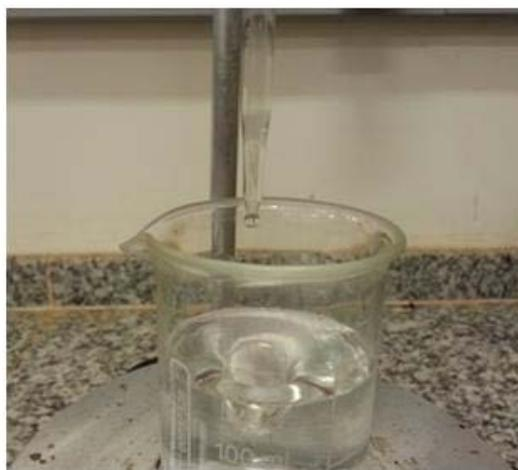
**Figure 1.** Slow drip of neutralizing solution for neutralization process of chitosan polycation.
