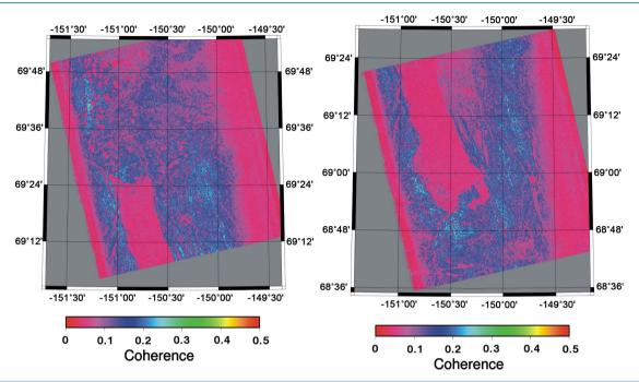
Figure 5. ALOS PALSAR InSAR coherence maps. Relatively higher coherence (surface scatters) occurs on rock outcrops (ridges and river bluffs) and low coherence (volume scatters) occurs on tundra vegetation active-layer.
