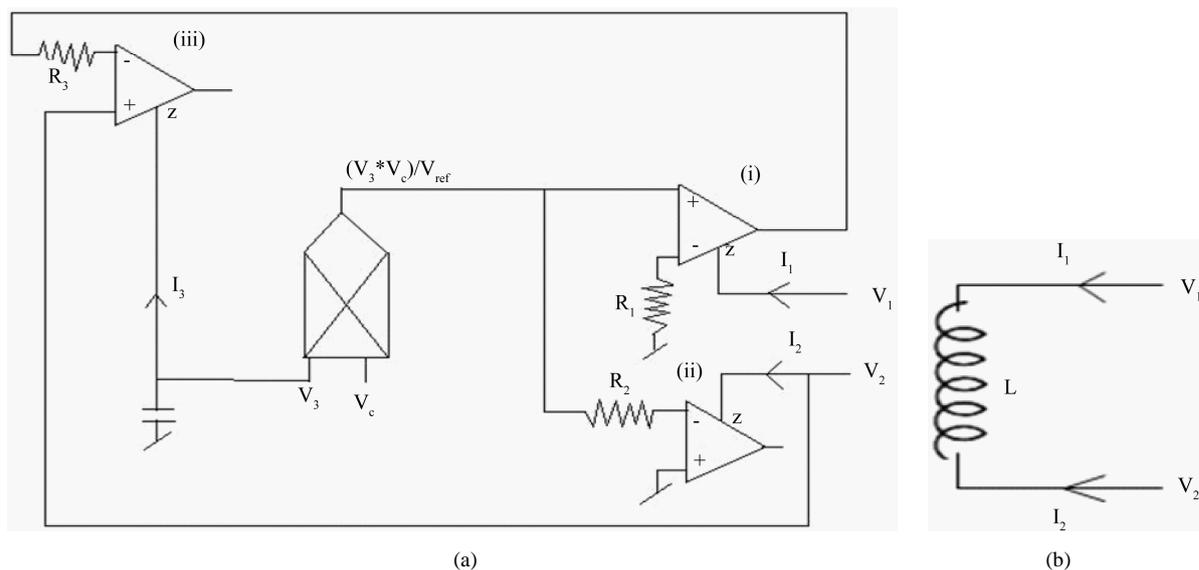
**Figure 3.** (a) Proposed floating linear voltage controlled inductance configuration; (b) Realized floating inductor.
