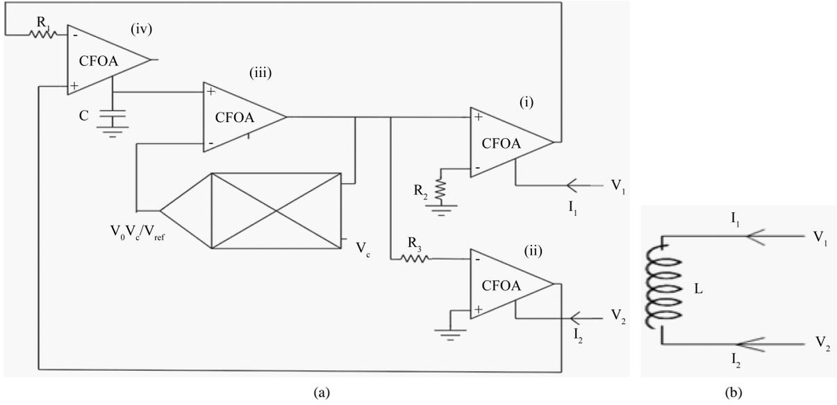
**Figure 2.** (a) Proposed floating voltage controlled inductance configuration; (b) Realized floating inductor.
