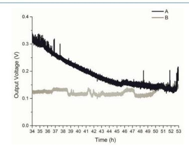
Figure 1. Response of output voltage in carbon cloth (A) and carbon brush (B) at the same stage.
