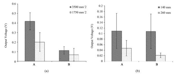
Figure 2. The output voltage of MFC in different projected areas. (a) and different distances (b). Vertical bars are means  $\pm$  S.D.
