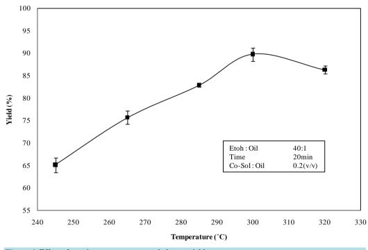
Figure 4. Effect of reaction temperature on ethyl ester yield.
