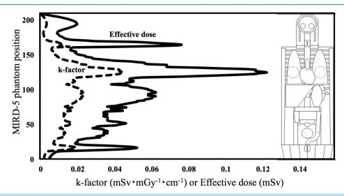
Figure 3. Comparison between different bolus tracking positions in terms of the effective dose and k-factor.
