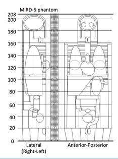
Figure 1. Schema for MIRD-5 phantom of ImPACT CT patient dosimetry. Measure shows the relationship between bolus tracking position and organ position.
