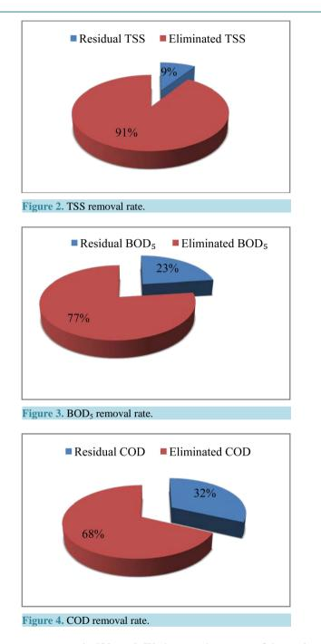
stable [12]. For COD, raw water content is 530 mg/l. We have at the output of the station the COD value which is equal to 172 mg/l with an efficiency of 68% (Figure 4) where the anaerobic tank provides 46%.
