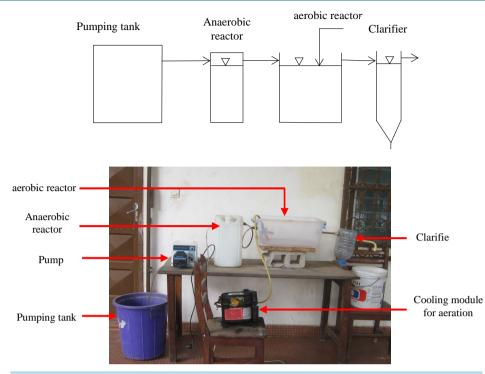
Figure 1. Anaerobic aerobic reactors.
