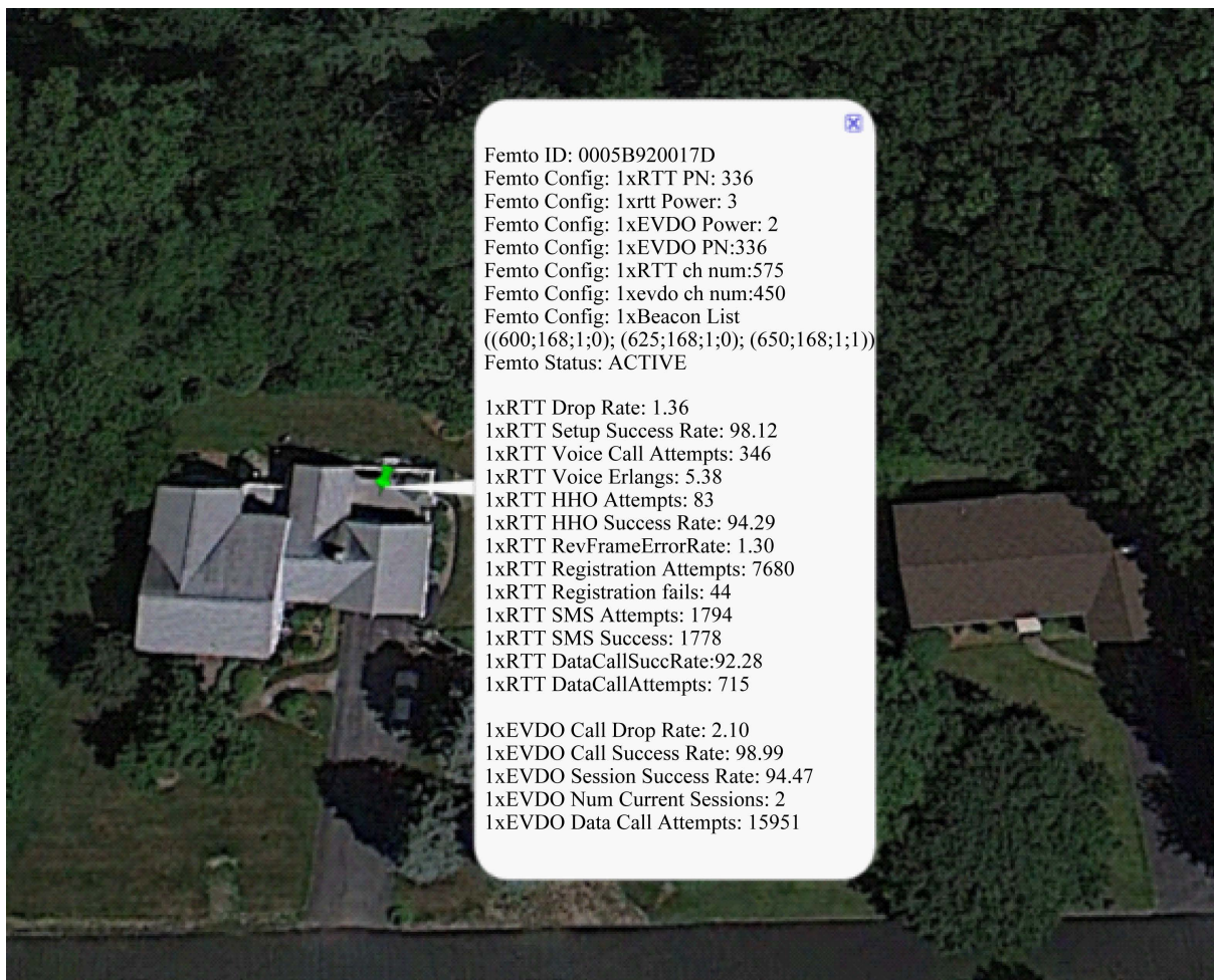
Figure 4. Graphical Interface showing performance and configuration of an individual femtocell over one month.
