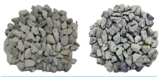
Figure 1. Batches of 19 mm recycled concrete and 19 mm natural aggregates.
