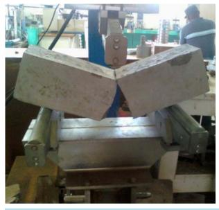
Figure 2. Typical flexural beam specimen failure.
