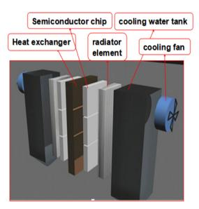
Figure 2. Cooling structure.
