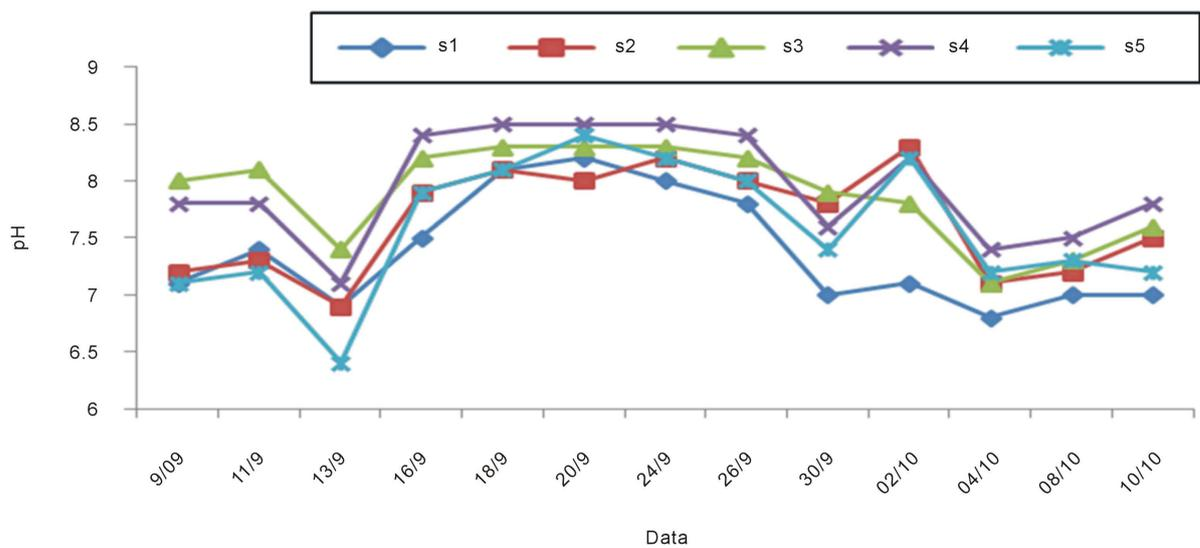
Figure 3. pH variations within the biogas digester.
