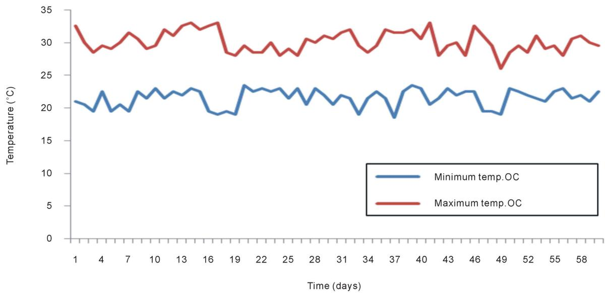
Figure 2. Temperature variation within the biogas digester.
