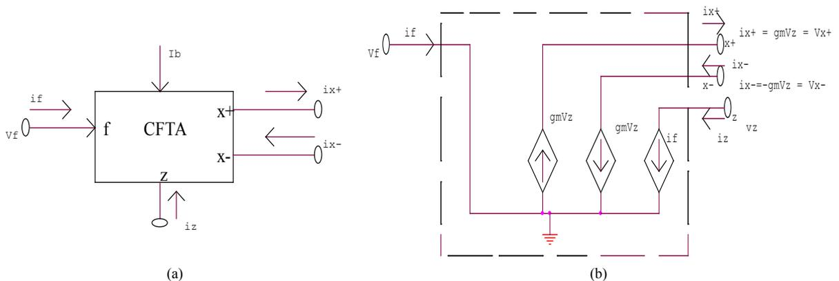
Figure 1. (a) The CDTA schematic symbol; (b) Behavioral model of CFTA.
