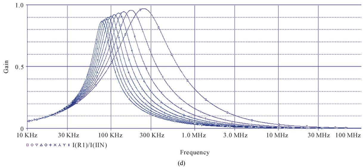
**Figure 4.** (a) Simulated frequency response of LP, HP, BP, and BR proposed CFTA current-mode second order biquad filter according to **Figure 2**; (b) Phase response of all pass proposed biquad filter; (c) Simulated frequency responses of the BP filter when  $Q_0$  is varied for  $f_0 = 245$  kHz; (d) BP filter with different  $f_0$  (keeping  $Q_0$  approximately constant).
