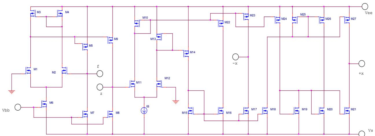
**Figure 3.** A CMOS implementation of CFTA used for simulations.
