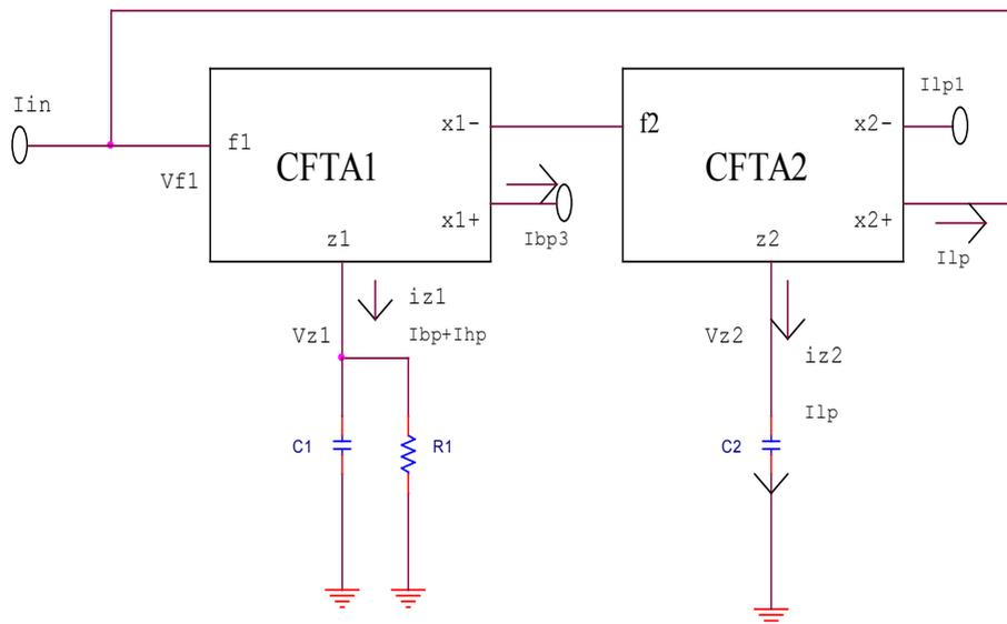
**Figure 2.** Proposed current mode second-order biquad filter using CFTAs.
