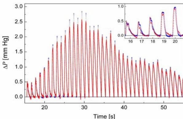
**Figure 6.** Plots of the pulsating part of the cuff signal (continuous curve) and the integral of the amplifier output signal after baseline subtraction (open circles). The inset shows the early part of the deflation phase (where the deviation between the two curves is most pronounced).
