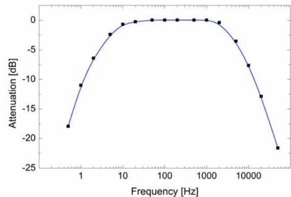
**Figure 2.** Frequency response of the filter-amplifier circuit.
