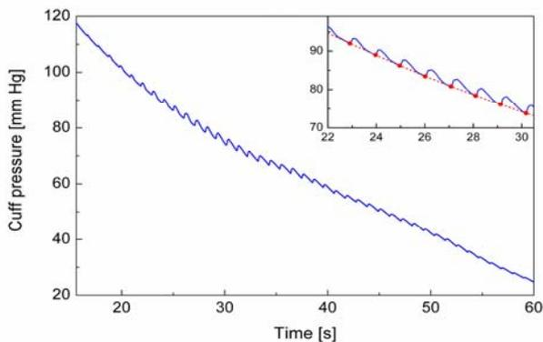
**Figure 4.** Plot of the direct output of the pressure sensor vs time (continuous line). The inset shows an enlarged portion of the main graph demonstrating the method of baseline subtraction. The local minima (filled circles) between each pulse were identified by a computer and interpolated to the whole region (dotted curve).
