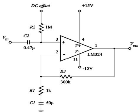
**Figure 1.** Circuit diagram of the oscillometric amplifier.
