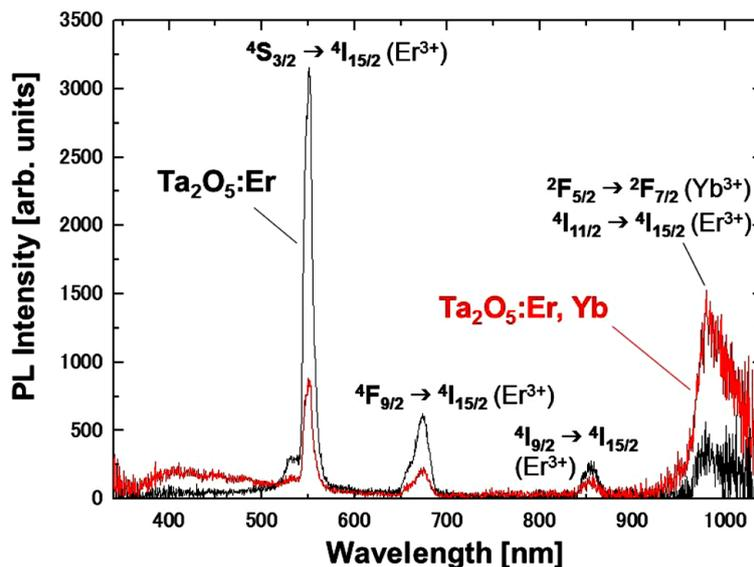
**Figure 2.** PL spectra of Ta<sub>2</sub>O<sub>5</sub>:Er, Yb and Ta<sub>2</sub>O<sub>5</sub>:Er [5] [6] co-sputtered thin films.
