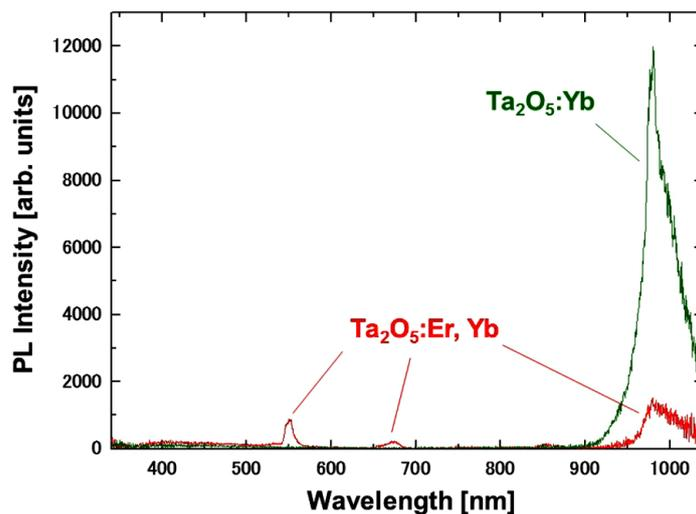
**Figure 4.** PL spectra of Ta<sub>2</sub>O<sub>5</sub>:Er, Yb and Ta<sub>2</sub>O<sub>5</sub>:Yb [7] co-sputtered thin films.
