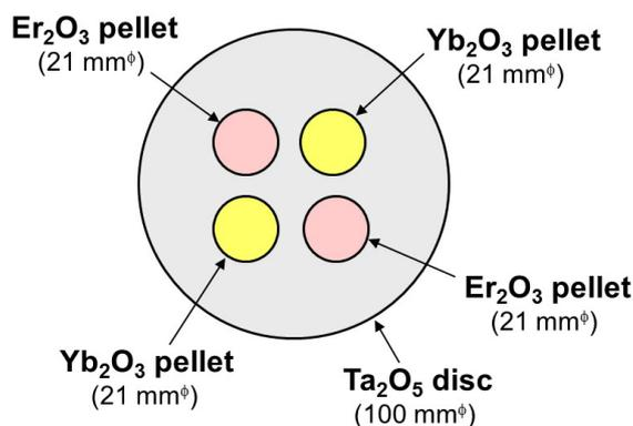
**Figure 1.** Schematic diagram of the sputtering target for co-sputtering of Er<sub>2</sub>O<sub>3</sub>, Yb<sub>2</sub>O<sub>3</sub>, and Ta<sub>2</sub>O<sub>5</sub> used in this work.
