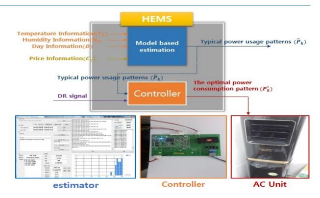
Figure 1. Layout of HEMS and setup environment.
