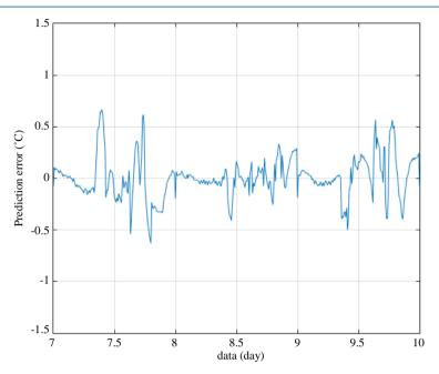
Figure 3. Prediction error (PE) for indoor-temperature.
