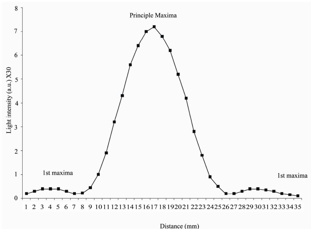
Figure 4. The relation between light intensity in (a.u.) and the traversed distance in (mm) to the left and right sides of the center of the principle maxima.)
