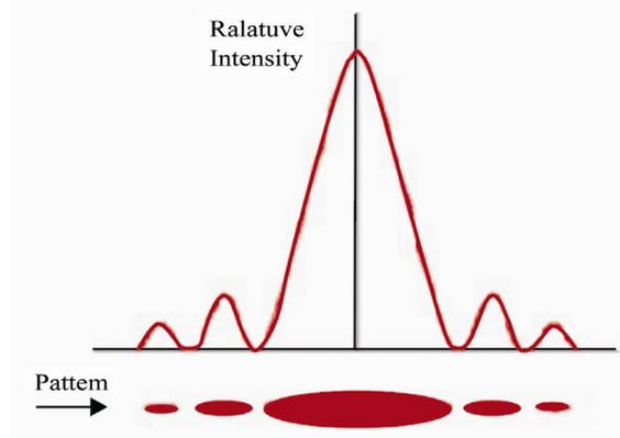
Figure 3. Single aperture diffraction pattern (Reproduced from: <http://www.saburchill.com/physics/chapters2/00081.html>-2010.
