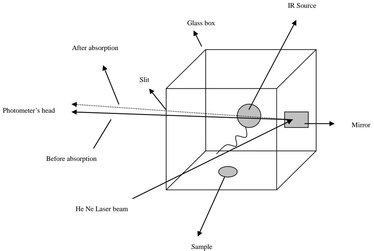
Figure 2. Schematic showing the PTLD experimental setup used to detect trace gas IR absorptions.
