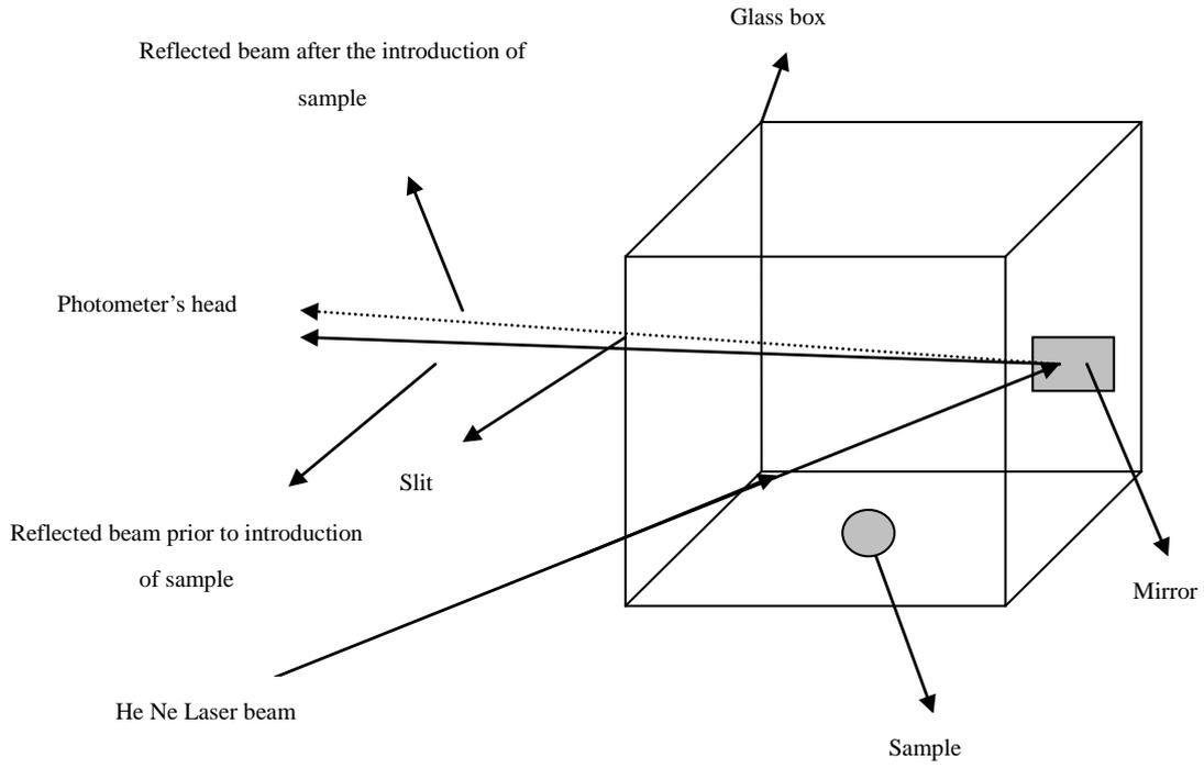
Figure 1. schematic showing the conventional Light Deflection cell used to detect gas trace emissions from different samples.
