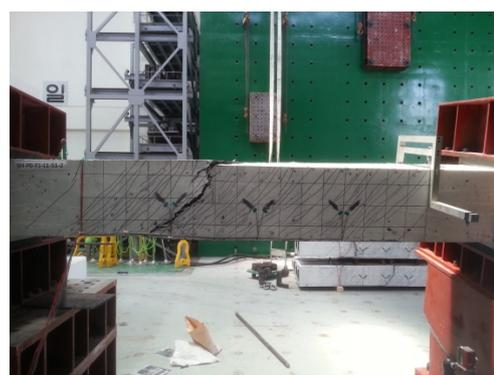
(b) Ultimate failure stage (SH-P0-F1-L1-S1(D13))(0 MPa prestress)
