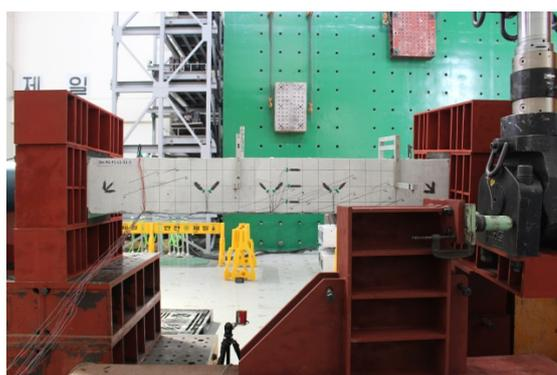
(a) Crack growth stage (SH-P4-F1-L1-S1) (50 MPa prestress)
