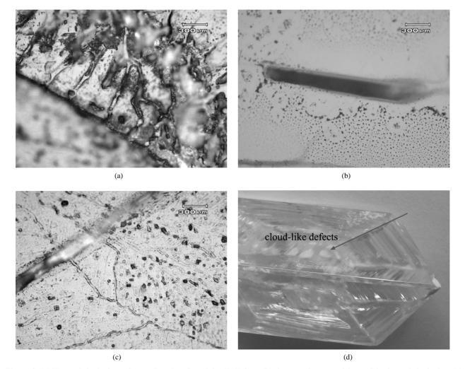
Figure 2. (a) The melt inclusions observed at the edge of the (110) face, (b) the negative crystal formed in the melt inclusion, (c) the inclusions containing insoluble particles with micrometer scale observed on the (200) faces, (d) cloud-like defects caused by large quantity of inclusions.
