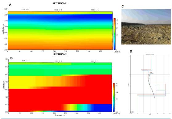
Figure 3. Interpretation of resistivity data at location 1 (a) TEM apparent resistivity pseudo-section; (b) TEM resistivity model cross section; (c) Site photograph; (d) Resistivity data log.
