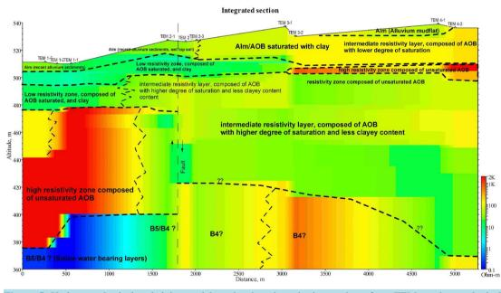
Figure 5. Hydro-geophysical resistivity model section based on the integration of ten TEM results, geological map, and geological cross section at Wadi Deir Al-Kahaf area.
