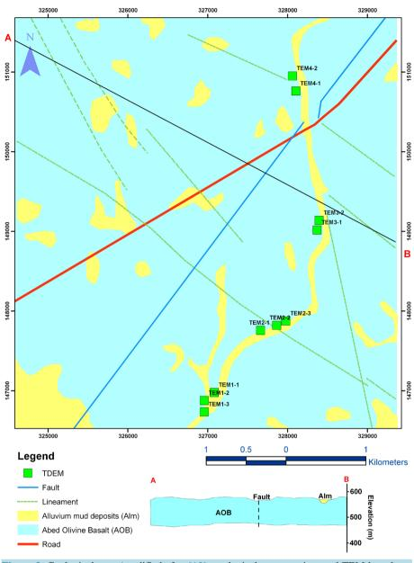
Figure 2. Geological map (modified after [13], geological cross section, and TEM loop locations at the study area).
