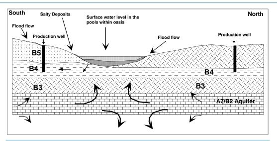
Figure 4. Schematic geological cross-sections through the Azraq area reveal subsurface hydrogeological condition along the study area, modified after [20] and [21].
