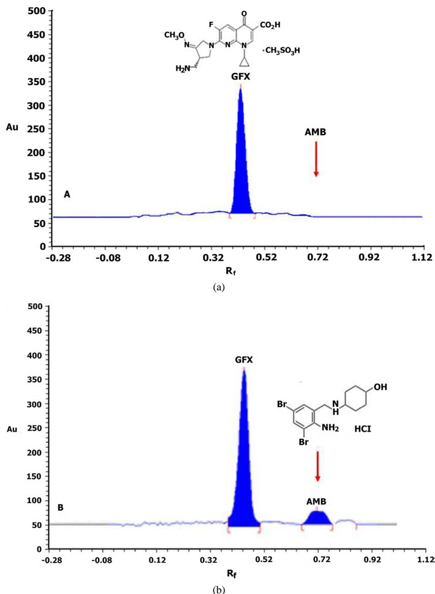
**Figure 2.** HPTLC densitograms of GFX (150 ng/band,  $R_f$  0.47  $\pm$  0.03) and AMB (35 ng/band,  $R_f$  0.72) using: (a) Fluorescence detection by optical filter K400 after excitation at 342 nm; (b) UV detection at 342 nm.
