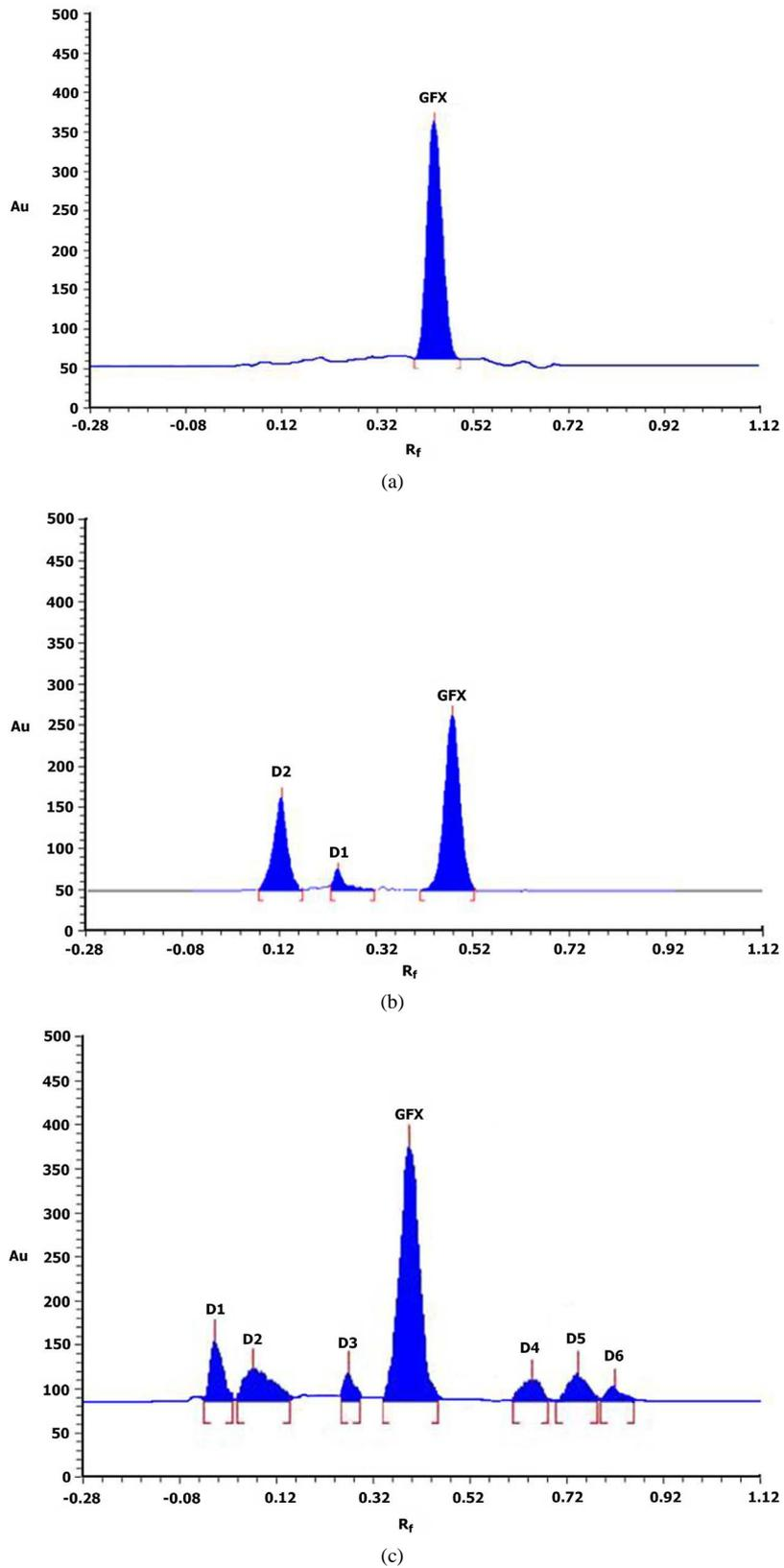
**Figure 3.** HPTLC densitograms of GFX (150 ng/band) at different stress conditions. (a) Pure GFX ( $R_f 0.47 \pm 0.03$ ); (b) Acidic; and (c) Photo-degradation conditions.
