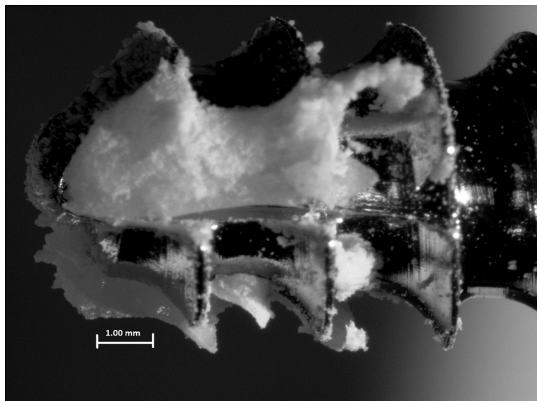
Figure 4. Photo of typical group B screw following removal with adherent cement in cutting flutes.
