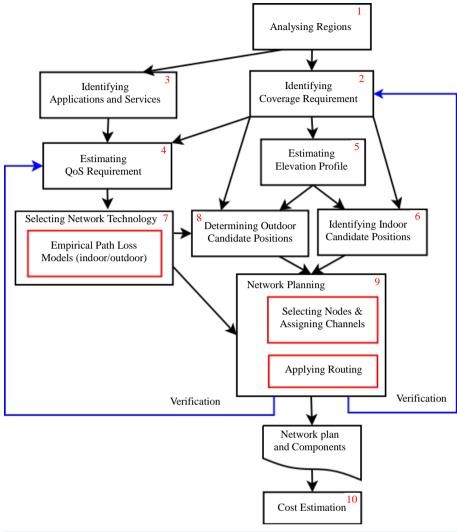
Figure 2. Design process model.
