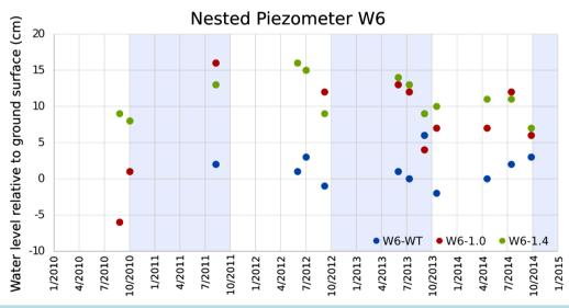
**Figure 12.** Water levels measured in the W6 piezometer cluster at Wilshire fen. Depth of the W6-WT piezometer was measured at 102 cm on 2-June-2012 (reported at 105 cm [4]). The piezometer was screened to 95 cm in peat. The W6-1.0 piezometers was measured at 104 cm bgs on 2-June-2012 (reported depth of 112 cm [4]). The W6-1.4 piezometer was measured at 144 cm bgs on 2-June-2012 (reported depth of 141 cm [4]).
