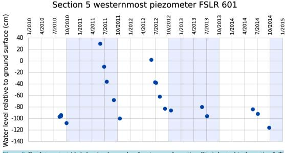
**Figure 9.** Depth to water table below local ground surface in a non-fen setting. Site is located in the section 5, T. 27 S., R. 10 E. (**Figure 2**) groundwater system. The thickness of the pumice deposit at this site was approximately 150 cm thick suggesting that most of the upper pumice unit had been eroded. FSLR = forest service local road.
