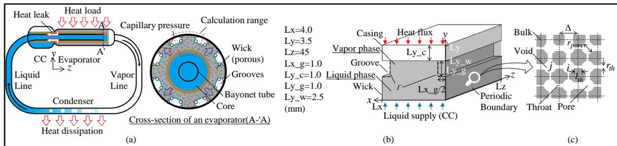
**Figure 1.** (a) Schematic of a loop heat pipe, (b) computational domain, and (c) representation of pore network model for fluid analysis in the wick.
