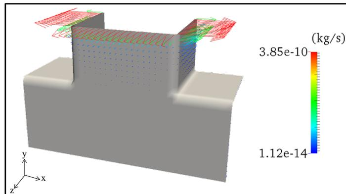
**Figure 8.** Mass flow rate on liquid-vapor interface viewed from rear.
