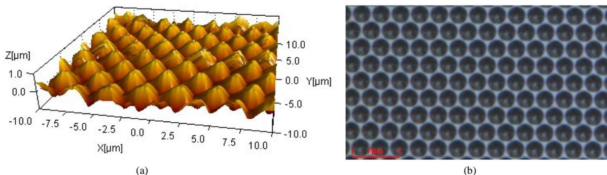
**Figure 1.** (a) AFM image of the PSS; (b) Optical microscopy image of the PSS.
