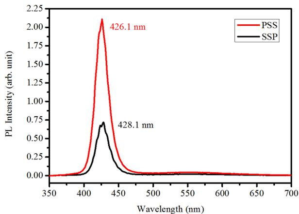
**Figure 2.** PL spectra of LED epitaxial structures on SSP and PSS.
