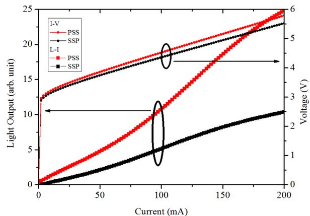
**Figure 4.** L-I and I-V characteristics of the LEDs on SSP and PSS.
