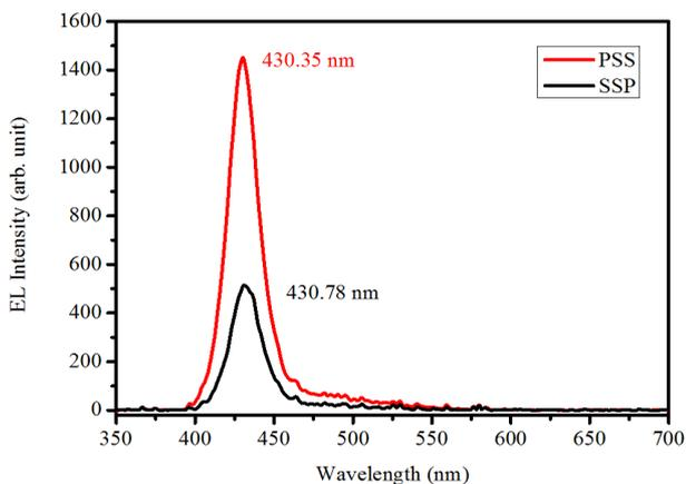
**Figure 3.** EL spectra of LED epitaxial structures on SSP and PSS.
