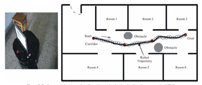
Figure 7. Performance demonstration of reactive navigation in a local environment using MT-R.
