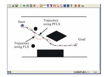
Figure 6. Simulated results of reactive navigation.
