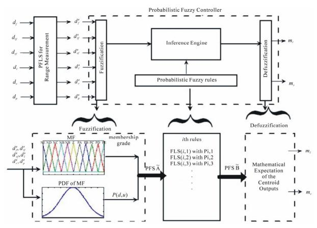
Figure 4. The PFLS controller for reactive navigation.
