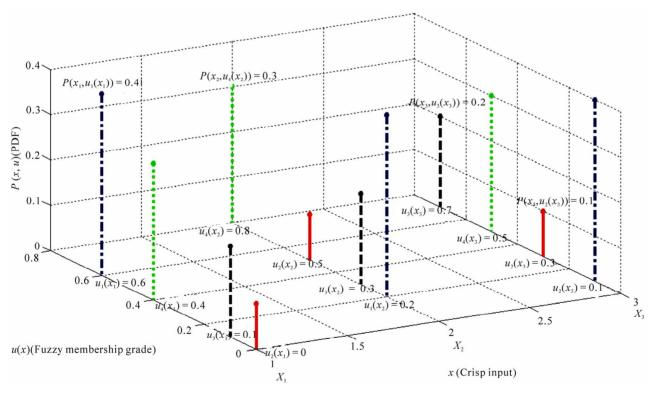
Figure 3. An instance of discrete probabilistic fuzzy set in three-dimension coordinate.
