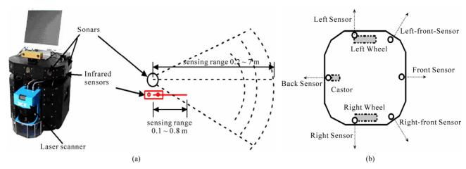
Figure 1. Mobile robot MT-R and its configurations. (a) MT-R mobile robot with rang sensors; (b) Configuration of Range sensors.
