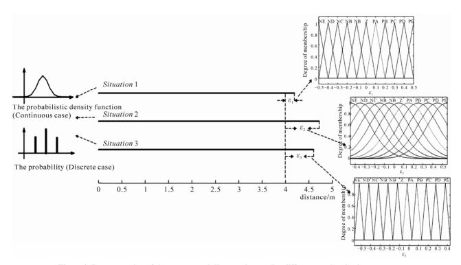
Figure 2. Demonstration of three measured distance data under different stochastic circumstances.
