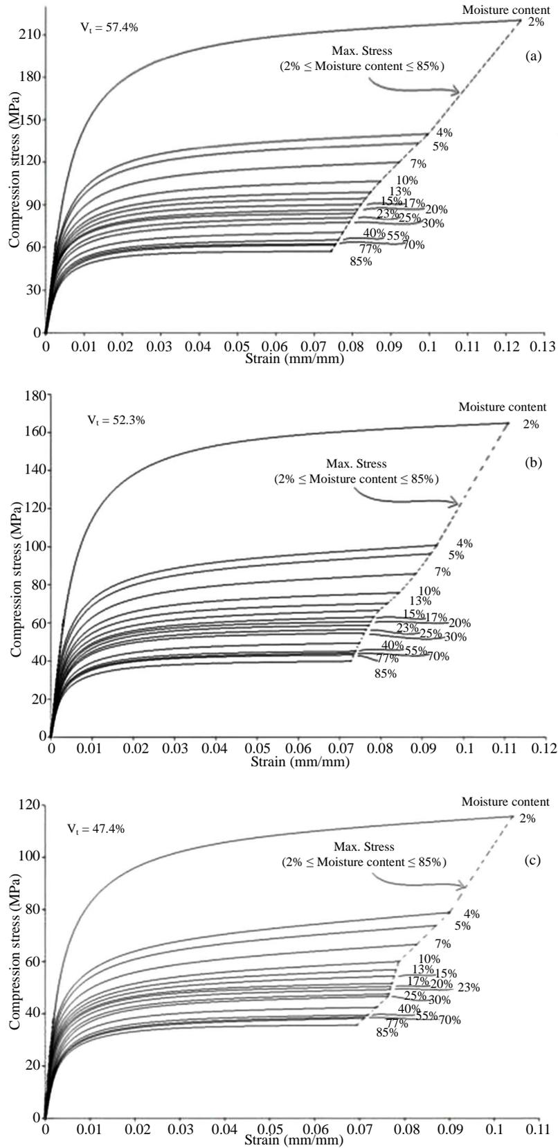
Figure 7. Moisture content effects on compressive stress-strain of DG bamboo.
