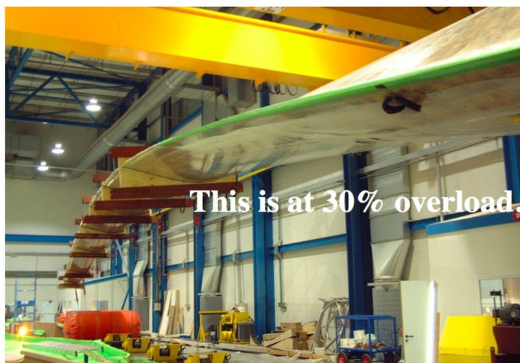
Figure 11. NEG Micon 40 m birch-wood/composite blade on test.
