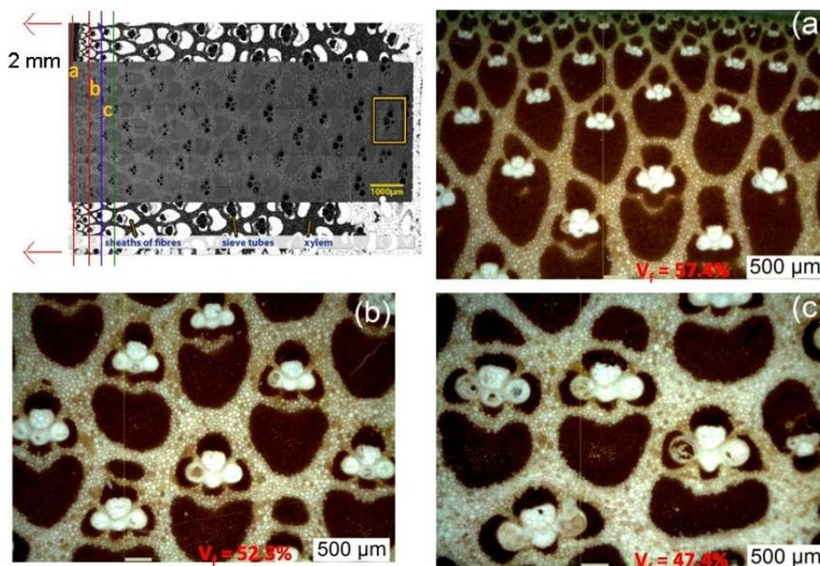
Figure 5. Outer wall fibre concentration in DG bamboo.
