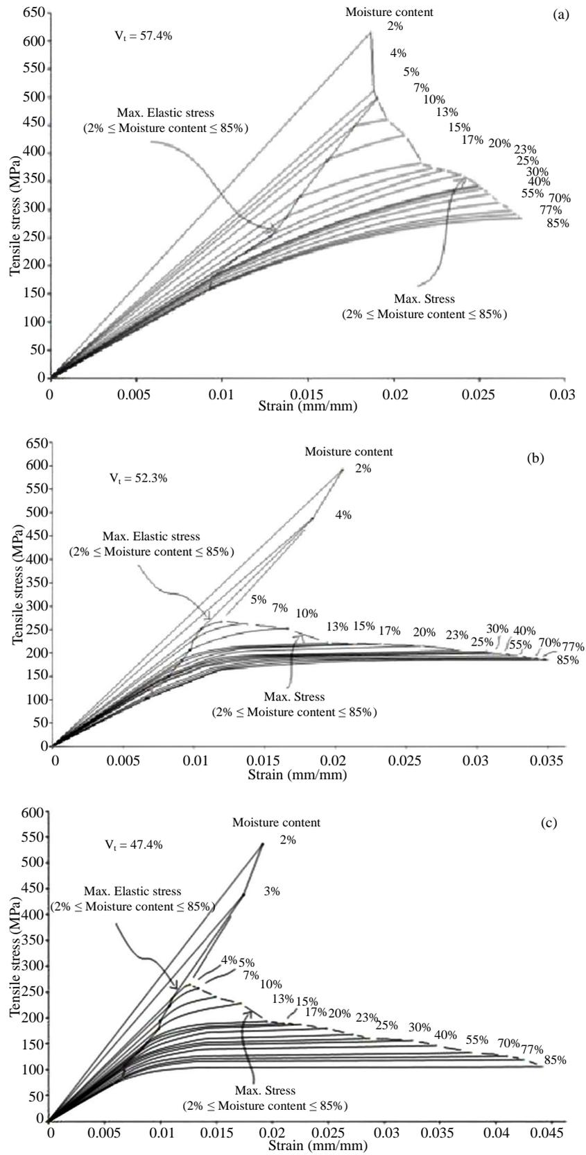
Figure 4. Moisture content effects on tensile stress-strain of DG bamboo.
