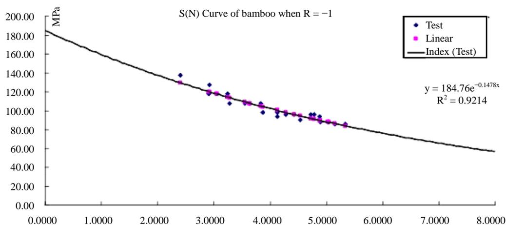
Figure 10. S(N) fatigue curve for Moso bamboo at R = -1.
