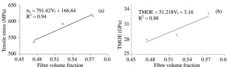
Figure 6. Tensile strength and stiffness variation with fibre volume fraction.
