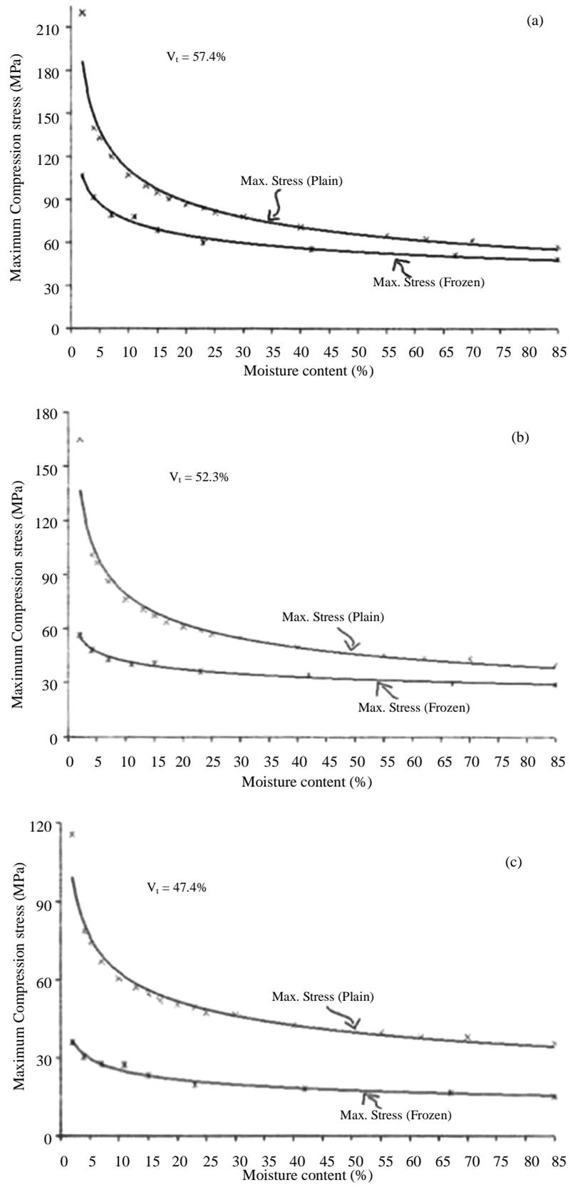
Figure 8. Loss of strength in frozen DG bamboo ( $-18^{\circ}\text{C}$ ).
