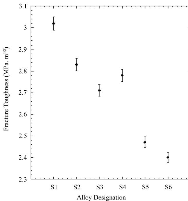
**Figure 4.** Fracture toughness against different Cr concentrations.
