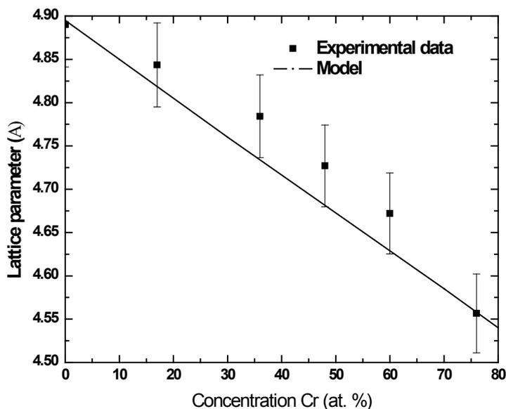
**Figure 5.** Lattice parameter as a function of Cr, experimentally and using the proposed model.
