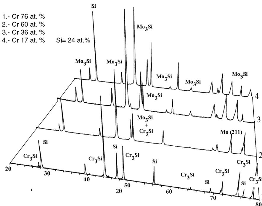
Figure 2. X-ray diffraction pattern from samples with Cr content.
