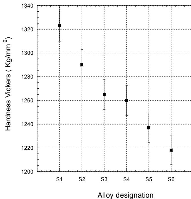
**Figure 3.** Microhardness as a function of Cr concentration.
