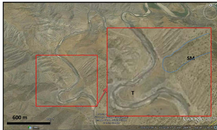
Figure 15. Google Earth image of a tributary of the Diyala River with horse shoe meander, due to landslide.
