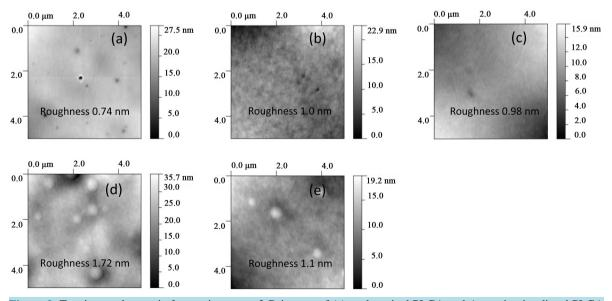
Figure 2. Tapping-mode atomic force microscopy 2-D images of (a) as deposited PLGA and Argon ion irradiated PLGA with doses (b)  $1 \times 10^{12}$  ions/cm<sup>2</sup>, (c)  $1 \times 10^{13}$  ions/cm<sup>2</sup>, (d)  $1 \times 10^{14}$  ions/cm<sup>2</sup>, and (e)  $1 \times 10^{15}$  ions/cm<sup>2</sup>.
