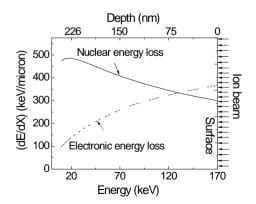
Figure 1. Illustration of 170 keV Argon energy loss within PLGA based on SRIM 2013 calculation.
