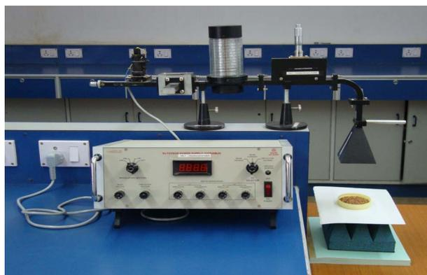
**Plate 1. Experimental set up for microwave exposure using Klystron based microwave test bench.**
