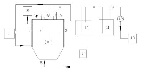
1. SC-15 water bath; 2. pH adjusting port; 3. organic reactor; 4. agitating blade; 5. reaction substrate outlet; 6. material inlet; 7. vent; 8. digital stirrer; 9. thermometer; 10. CO2 removal; 11. desiccant; 12. wet gas flowmeter; 13. GC-7900 gas chromatography; 14. nitrogen purging port.
