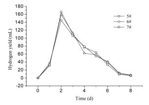
Figure 6. production hydrogen of anaerobic digestion from sludge by heat digestion.
