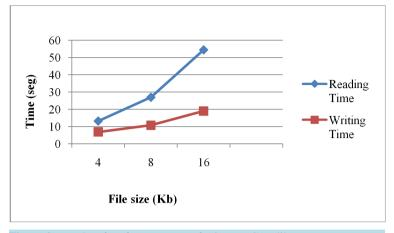
Figure 9. Results of performance tests for iButtonCom library.
