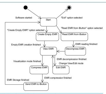
Figure 4. State diagram for the EMR managing system.
