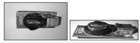
Figure 7. Hardware interface for exchanging information between a PC and the iButton.
