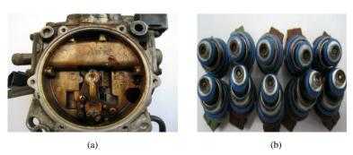
Figure 1. The contamination in vaporizer and injector from LPG vehicles. (a) Vaporizer contamination; (b) Injector contamination.
