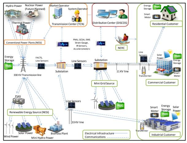
Figure 7. The proposed smart grid system.
