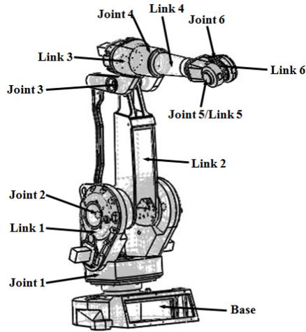
Figure 1. The three-dimensional model of the 6R robot.
