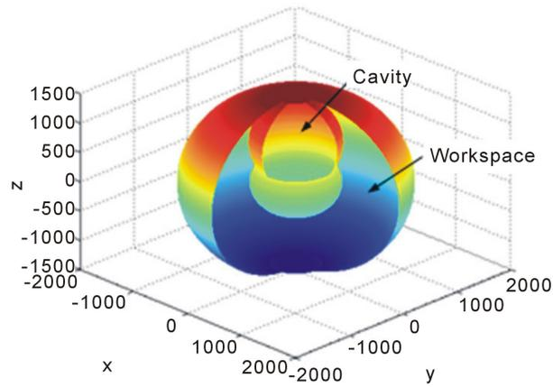
**Figure 5.** The three-dimensional cross-section view of the workspace.
