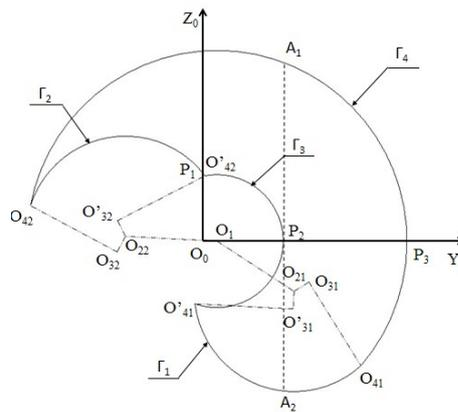
Figure 3. The section shape of the workspace of 6R robot on the  $X_0O_0Z_0$  plane.
