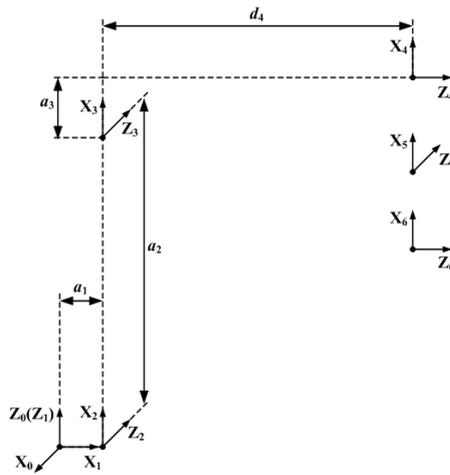
Figure 2. The D-H coordinate frames of the 6R robot.
