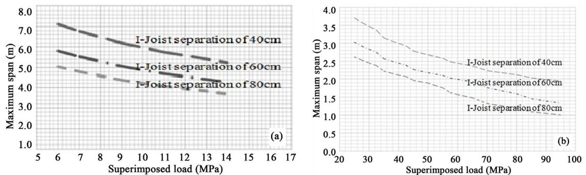
Figure 5. Maximum span in I-joist fabricated with bamboo's flanges for use in (a) flooring and (b) roofing.
