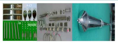
Figure 2. Standard capsule, parts and specimens.
