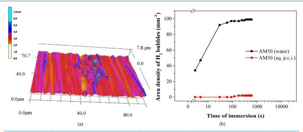
**Figure 6.** (a) Laser Scanning Confocal Microscopy (LSCM) image of a freshly emeried AM50 surface, and (b) incidence of hydrogen bubbles on AM50 samples immersed in clean water and, respectively, an aqueous polymeric corrosion inhibitor (p.c.i.) formulation as a function of immersion time.
