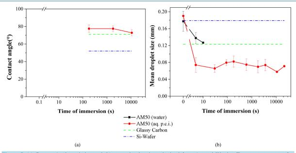
Figure 5. (a) Contact Angle variation and (b) mean droplet sizes obtained from Aerosol Wetting Test measurements after different immersion times in clean water and in an aqueous p.c.i. formulation, respectively.
