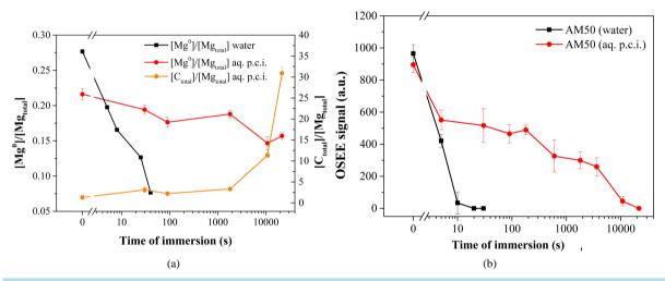
**Figure 7.** Effects of immersing AM50 in clean water and, respectively, a formulation of polymeric corrosion inhibitor (p.c.i.): (a) Concentration ratios of  $[Mg^0]/[Mg_{total}]$  and  $[C_{total}]/[Mg_{total}]$  as function of immersion time, obtained by XPS; (b) OSEE signal as a function of immersion time.
