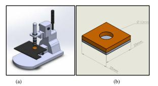
**Figure 3.** Sketches displaying the experimental procedure of the Hydrogen Bubble Formation Test ( $H_2BT$ ); (a) Set-up with sample on microscope table; (b) metal sample with silicone mould on top.
