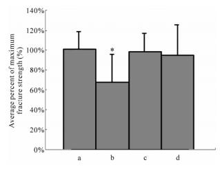
**Figure 3.** The average percent of maximum fracture strength of silk fibroin unsterilized (a), and sterilized using steam (b), gamma irradiation (c), and ethylene oxide (d) (n = 6). \*p < 0.05 versus the unsterilized group.
