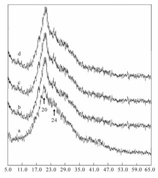
**Figure 2.** X-ray diffraction curves of unsterilized silk fibroin (a) and silk fibroin sterilized using steam (b), gamma irradiation (c), and ethylene oxide (d).
