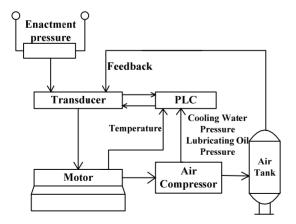
Figure 2. System schematic diagram
