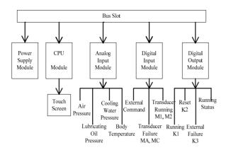
Figure 5. Configuration of the PLC
