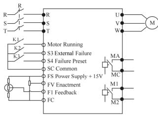
Figure 4. Connection circuit of the transducer
